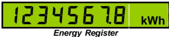
Scaling of the energy register is set by the nominal input currents and voltages and remains constant during operation of the meter.
